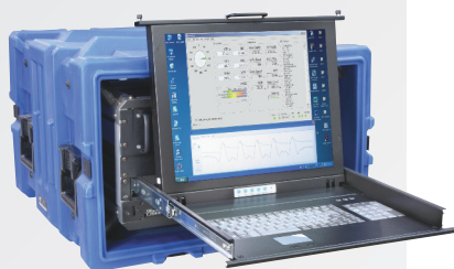
SureShot Ruggedized System with Integrated Server and Terminal
