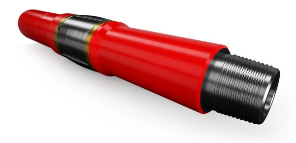
The Runner™ is an integral drill string component consisting of a short one piece mandrel that utilises proprietary bearing technology to support a non-rotating one piece sleeve. The tool is positioned between connections of the drill pipe and spaced appropriately throughout the build section of the wellbore or formation generating the string torque.
